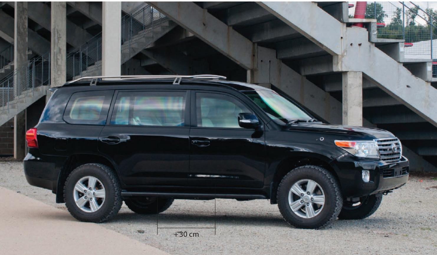
**S**tretched by 30 centimeters at the rear doors. The original lines are respected. These Carat Duchatelet armoured vehicles bring class and exemplary discretion whilst traveling.
