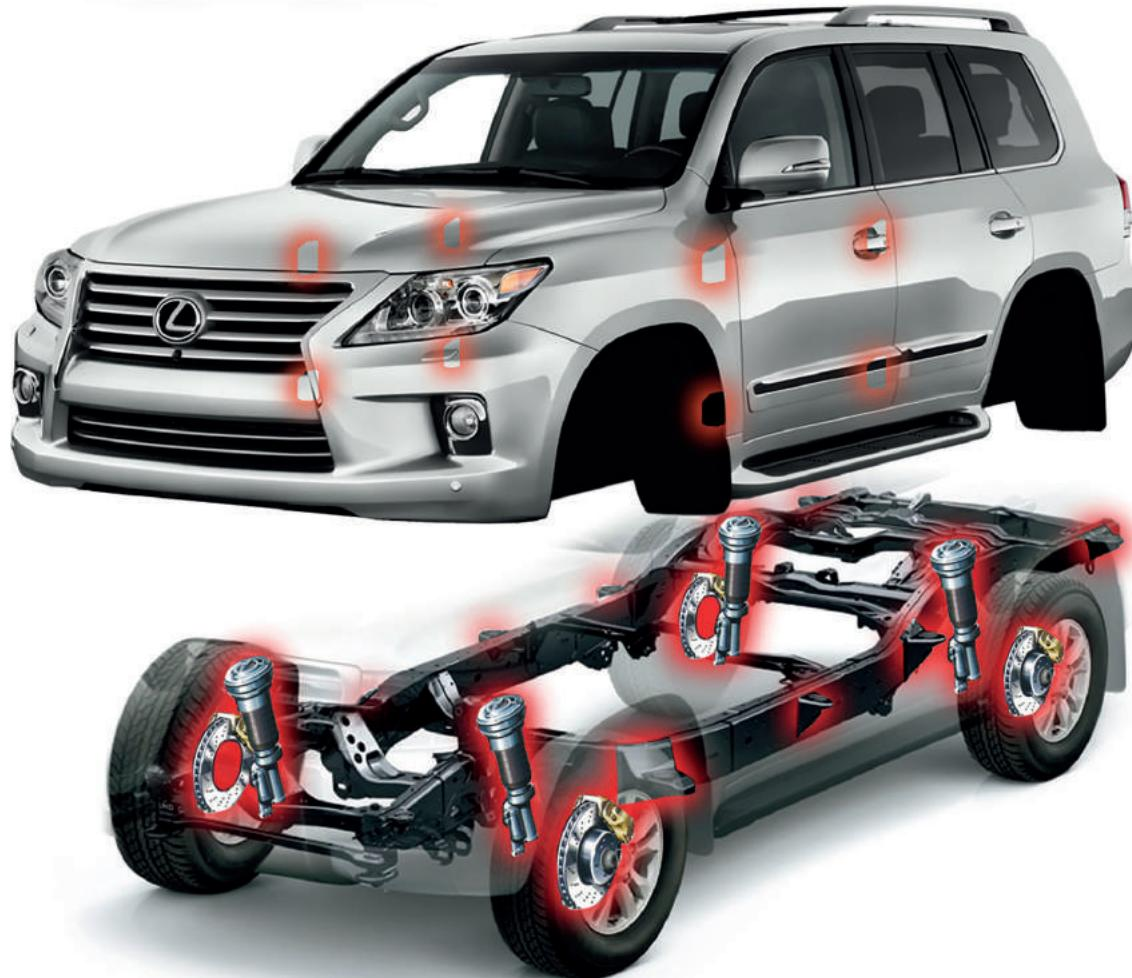
To ensure durability and off-road capabilities despite a higher weight, we paid particular attention to strengthening links between frame and body. New suspensions were also studied in order to face the most extreme conditions. Suitable brakes enable braking with original performance. All these elements are essential both for the longevity of the vehicle and its ability to extricate you from any situation.
